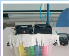
The small but mighty prototype demonstrated evaporative cooling of the air.
